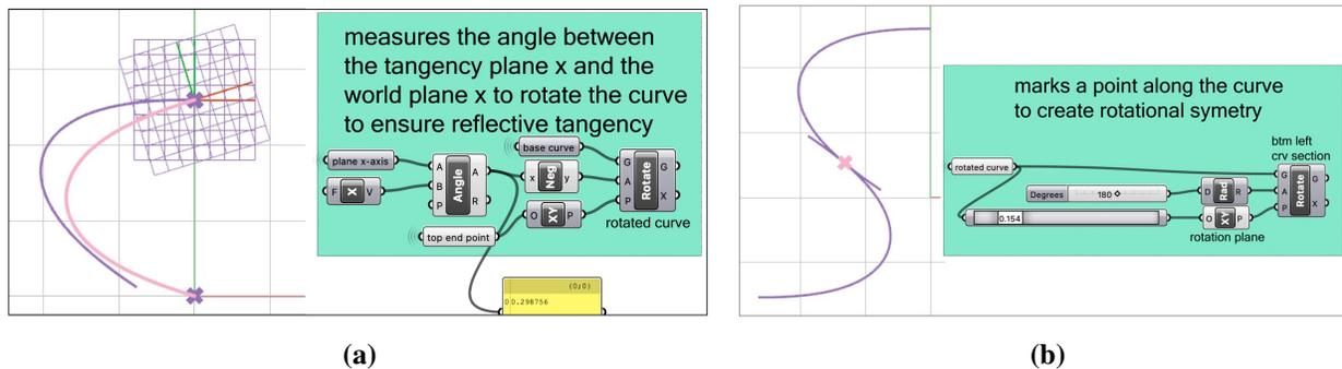
**Figure 3:** The catenary curve is rotated to tangent (a), and is rotated 180-degrees from a point along the curve for rotational symmetry (b).
