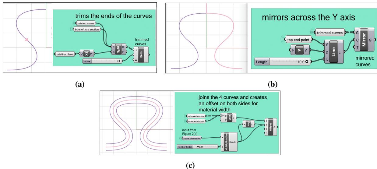
**Figure 4:** The curves are trimmed at the point of rotation (a) and both segments are mirrored across the Y-axis (b). The curves are joined and offset (c).
