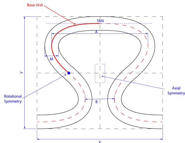
**Figure 1:** *The basic geometric considerations of a single stitch of knitting.*
