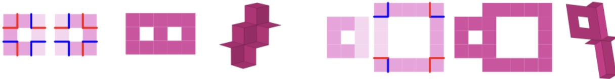
**Figure 5:** On the left, a closable  $2D$ -*patching* of two  $1 \times 1$  square fenestrations. We highlight the folding patterns that are compatible. On the right, a non-closable polyomino built from  $2D$ -*patching* a  $1 \times 1$  and a  $3 \times 3$  square fenestration.
