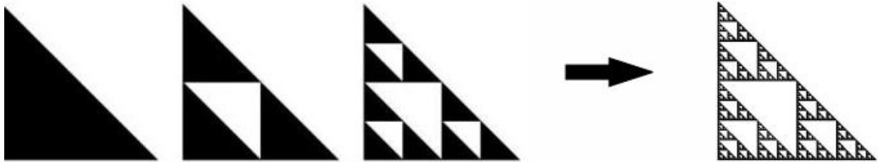
Figure 1: Initiator, generator, and approximations leading to the Sierpinski gasket.
