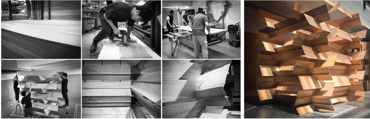
Figure 5: Teaching-based exercise for reversible connections using diagonal cutting slots.
