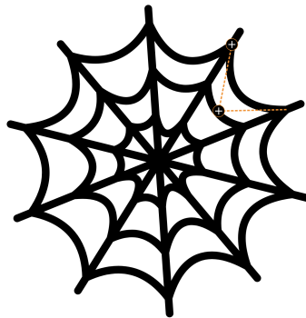
Figure 6: A spider web made of rings of quadratic Bézier curves, with one selected for direct manipulation.
