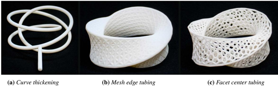
**Figure 6:** 3D-printed  $(3,2)$  torus minimal surface with different mesh postprocessing effects
