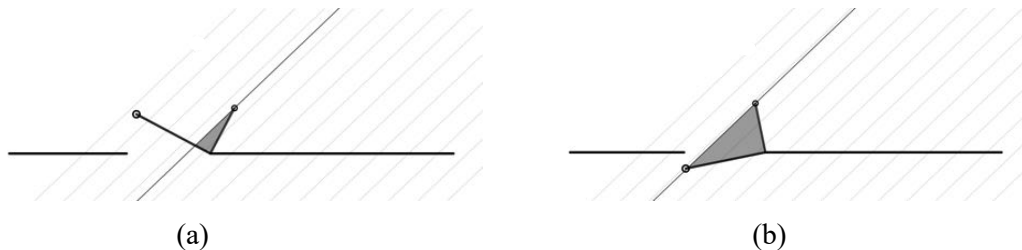
Figure 3: (a) Tilting the shadow plane toward the Sun increases apparent altitude/shortens shadows (multiplier is less than 1), (b) tilting the shadow plane away from the Sun decreases apparent altitude/lengthens shadows (multiplier is greater than 1)
