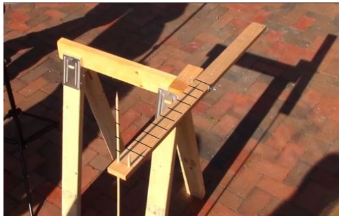
Figure 1: Prototype of the SunRule. Rulings on the orthogonal rods are equal to those on the board. Rulings emphasized to aid visibility. In the figure, the unit shadow (shorter rod, multiplier) is 2, the multiplicand (taller rod) is 5, and the length of the multiplicand's shadow is 10—i.e., 2 \times 5 = 10 .
