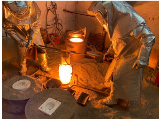
Figure 6: Casting bronze for the ball-and-socket; left: fourth author, right: first author.
