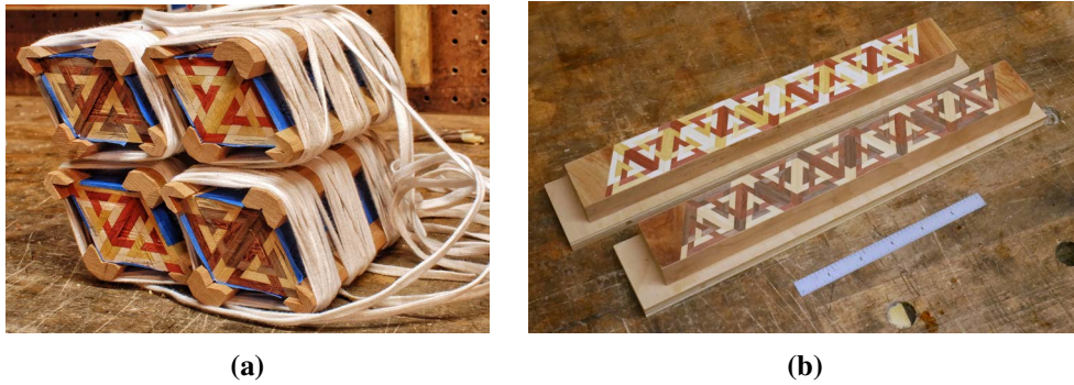
Figure 5: Assembling the cells into the final pattern block. (a) Arranging the cells into intermediate parallelogram blocks, (b) the two final Borromean rings pattern blocks.
