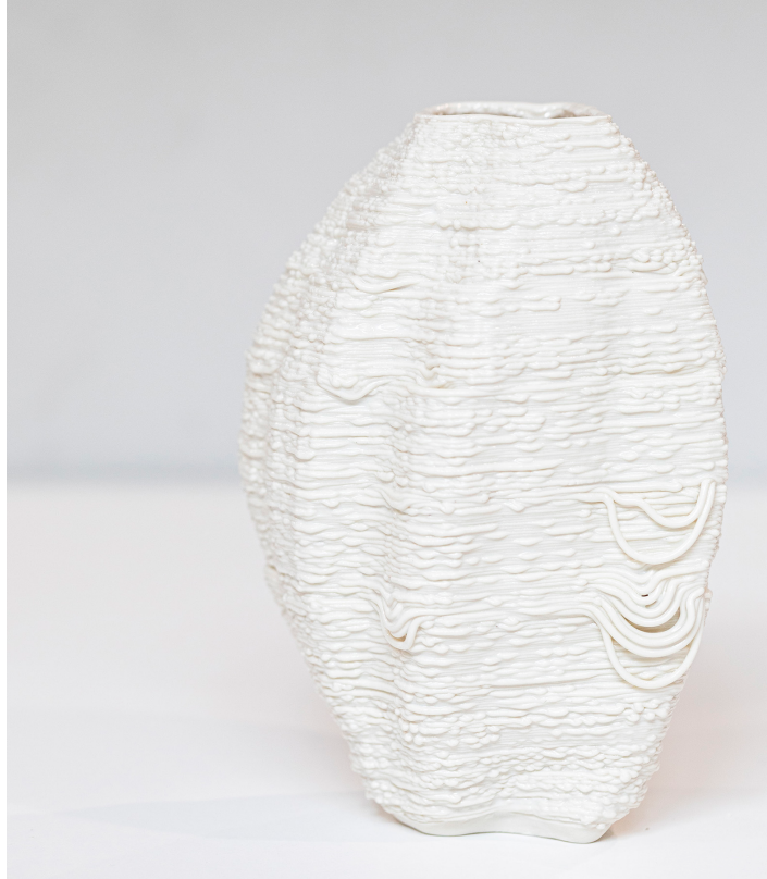
Figure 3: Sections of the perimeter create smaller or larger “dropped” loops of clay. These are unpredictable glitches of code and clay, which make printing with the material somewhat unpredictable and filled with exciting potential.
