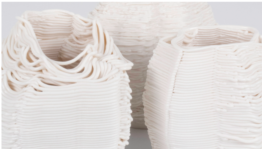
Figure 1: Examples of 3D printed porcelain using the Pathfinder code. The basic shape is the same, while the surfaces vary depending on the algorithm settings and on glitches of the code or printing.
