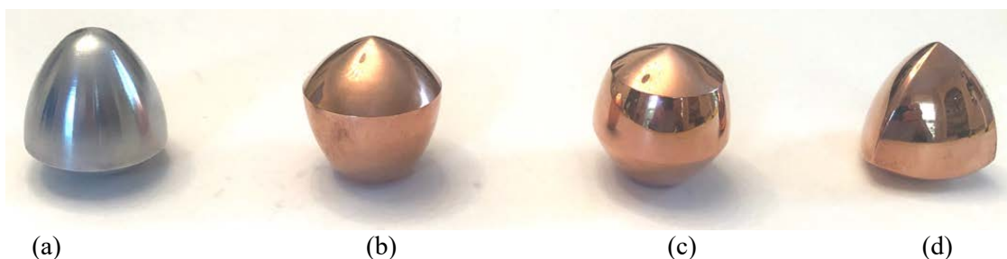
Figure 4: (a) Reuleaux, (b) pentaorbiform, (c) heptaorbiform, and (d) tetraorbiform (each ~ 5 cm).
