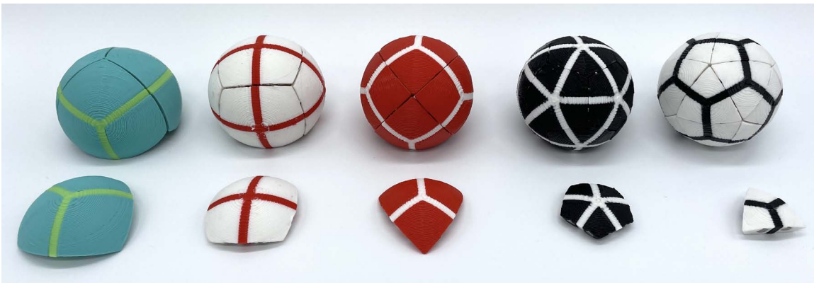
Figure 2: The five self-assembling spherical Platonic solids are 3D-printed to visually represent their duals, with an individual component displayed in front. Left to right: The Tetrahedron, Cube, Octahedron, Dodecahedron, and Icosahedron
