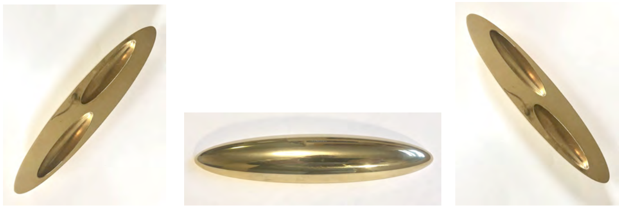
Figure 5: Top view of right and left handed brass \delta CELTs and bottom view (15.2 cm x 3.2 cm x 1.6 cm).
