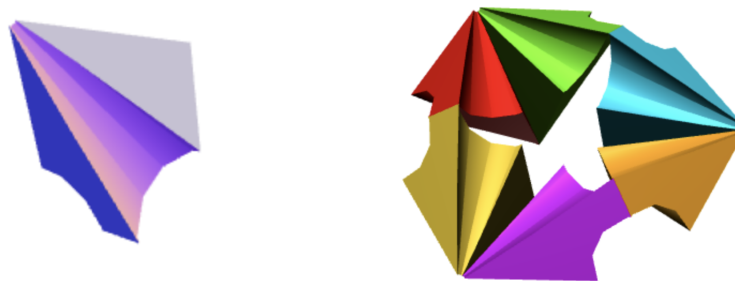
Figure 7: Left: a cell from a n = 6 kaleidocycle after undergoing two conical cuts along its edges; right: an n = 6 kaleidocycle built from the cell.
