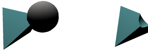
Figure 4: left: a spherical tool overlapping a cell's vertex; right: a new cell created after a subtraction operation
