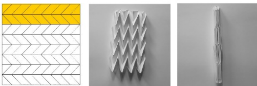
Figure 1. A Miura-ori and its folded forms.
