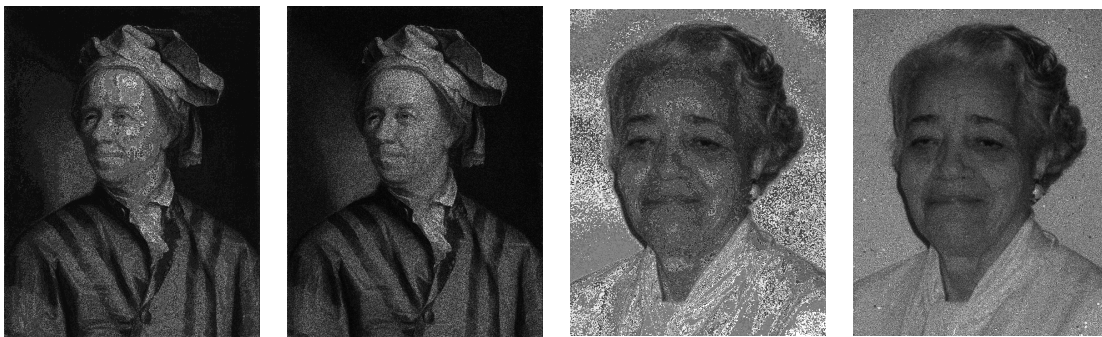
Figure 2: Totient transforms at N_H = 50 and N_H = 250 of the grayscale Euler and Vaughan images.
