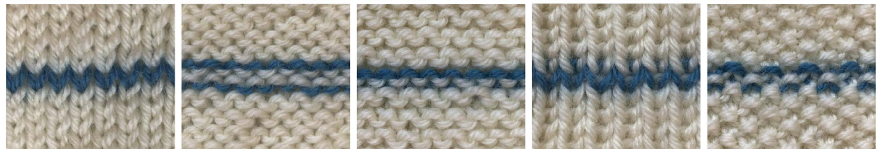
(a) Stockinette fabric is formed by a lattice of knit stitches. (b) Reverse stockinette fabric is formed by a lattice of purl stitches. (c) Garter fabric alternates rows of all knit and all purl stitches. (d) 1×1 ribbing alternates columns of all knits and all purls. (e) Seed fabric is a checkerboard lattice of knits and purls.
