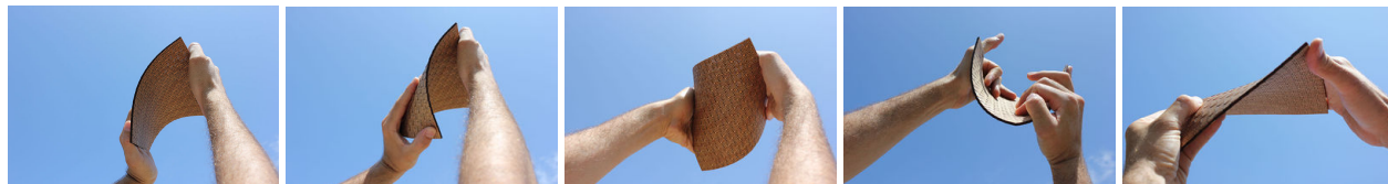
Figure 2: Highly flexible plywood obtained by relief cutting by 2D meander pattern invented by Dujam Ivanišević (Images courtesy of Dujam Ivanišević).
