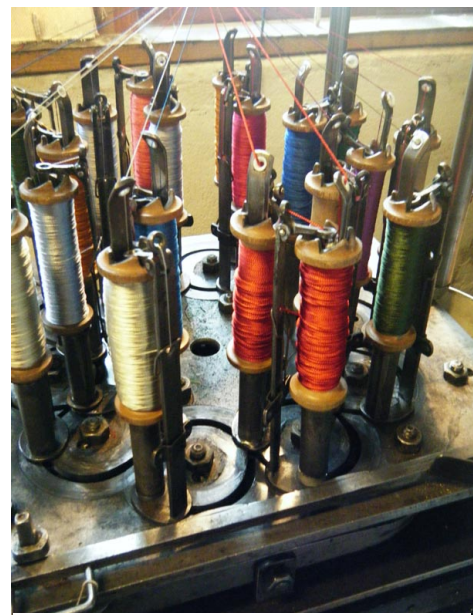
Figure 3: ‘Dancing’ bobbins on braid machine (E. Knoll)
