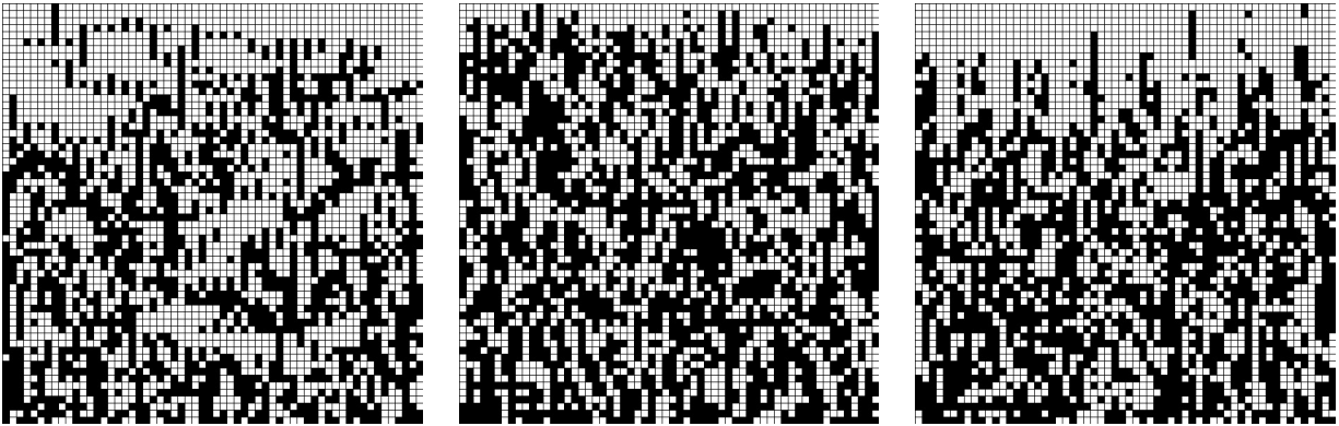
Figure 3: Variations of the ballistic deposition model when the grid resolution is 60 \times 60 and where the neighboring columns considered are w columns distant when (left to right) w = 2 , w = 5 , and w = 8 .
