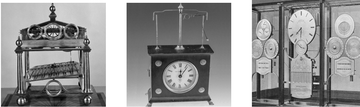
Figure 1: Curiosity clocks: Inclined plane clock, flying pendulum clock and Jens Olsen's astronomical clock at Copenhagen town hall.
