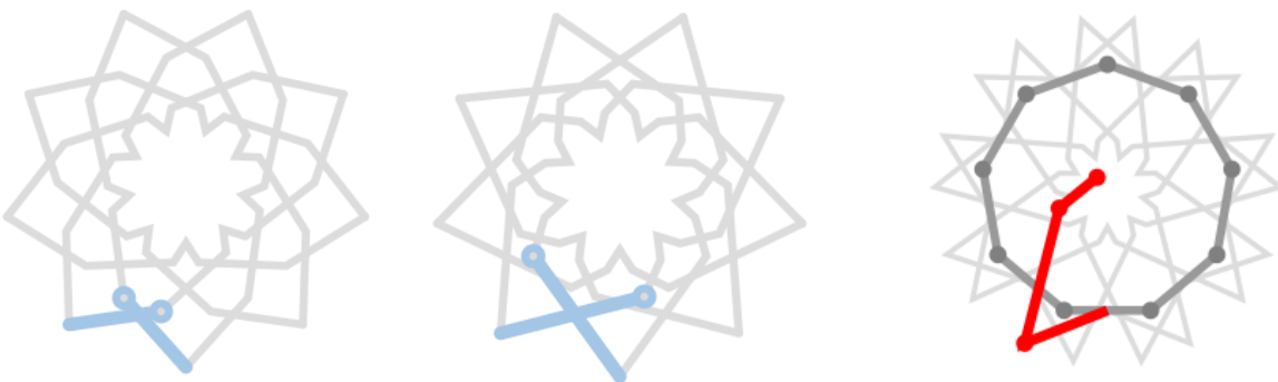
(a) Pattern vertices may cross each other during optimization, causing the pattern structure to be qualitatively different. (b) Optimization may move control points beyond tile boundaries.
