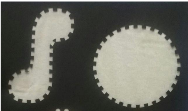
Figure 5: Two laser cut planar shapes with notches.
