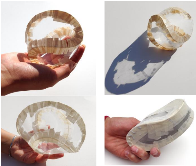
Figure 7: Examples of D-form surfaces used for casting.
