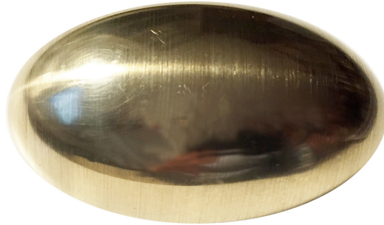
Figure 3. A brass version of the \Phi TOP with major axis \sim 5.1 cm, weighing \sim 220 grams.
