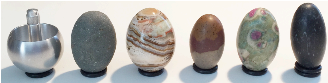
Figure 1 (from left to right): (a) aluminum tippe top; (b) natural pebble; (c) polished agate stone egg; (d) classic Lingam stone; (e) ruby/fuschite Lingam stone; (f) black Lingam stone. Each is about 5 cm tall.
