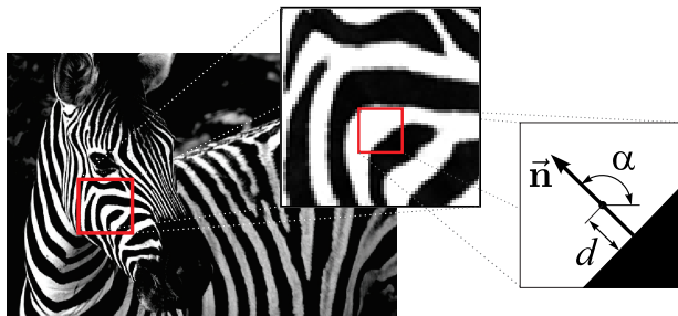
Figure 1: An example of a natural image. Sufficiently small patches of the image can be well approximated with just a pair of parameters.
