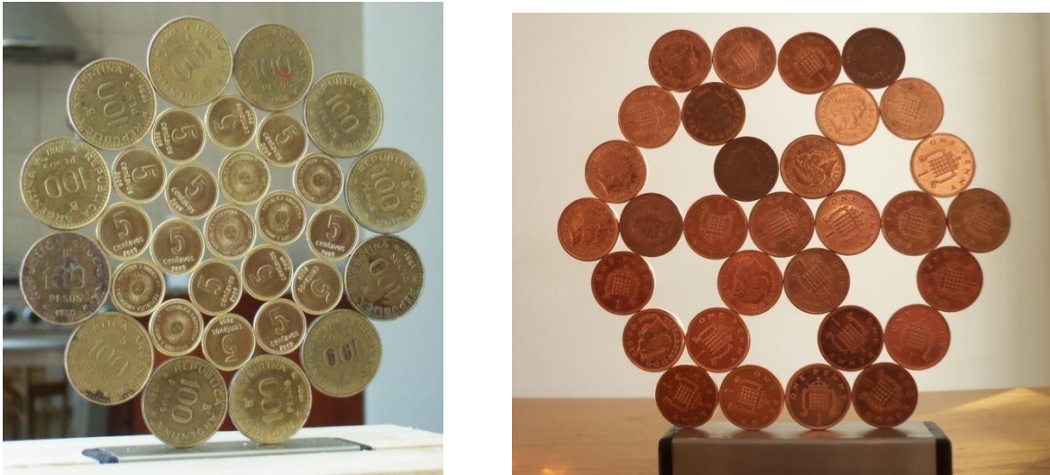
Figure 6. Standing hexagonal arrays illustrating the power of magnetic fields and the mechanical triangle-like rigidity resulting from three circle contact.
