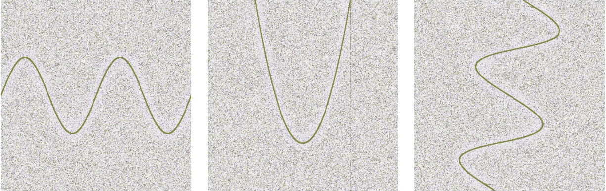
Figure 4: Cartesian curves used as target curves. Left: The sine curve y = a \sin(bx) with a = 100 , b = \pi/125 . Middle: The parabola y = ax^2 - b with a = 3/125 , b = 125 showing an out of range example. Right: The sine curve y = a \sin(bx) with a = 100 , b = \pi/125 rotated about the local origin by 4\pi/9 radians.
