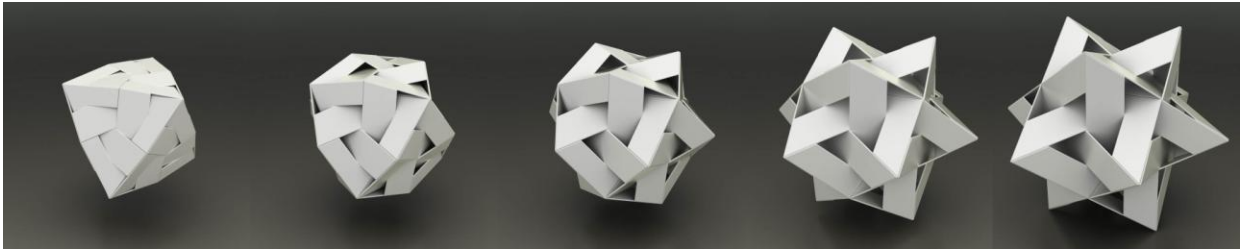
Figure 17: Development of the shape of the faces of the second stellated icosahedron.
