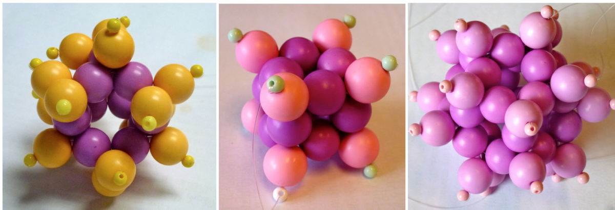
Figure 2: Bead valence sphere models of adamantane ( C_{10}H_{16} ), cubane ( C_8H_8 ), and dodecahedrane ( C_{20}H_{20} ).
