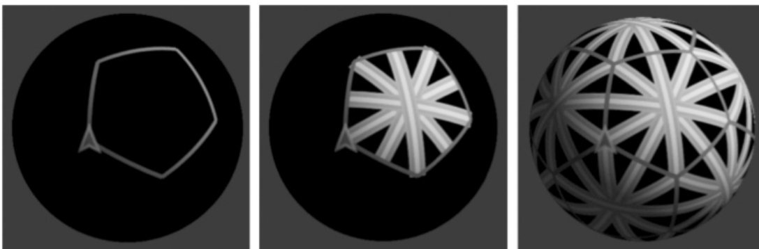
Figure 8. Left: a dodecahedral pentagon, drawn in blue. Center: Interior lines added to the pentagon. Right: the pattern at the center repeated over the entire sphere.
