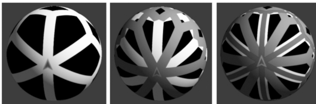
Figure 5. Left: two inscribed cubes, offset by 60 degrees. Center: Six pair of broken red lines are added (a similar set of six pairs is drawn opposite on the sphere). Right: the original cube structures are redrawn in blue.
