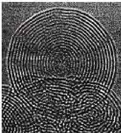
Figure 6: High resolution transmission electron microscope image of an onion-like spheroidal carbon particle. Flattening of the shells is most obvious in the outer arcs between 8 o'clock and 11 o'clock. Image by Daniel Ugarte.
