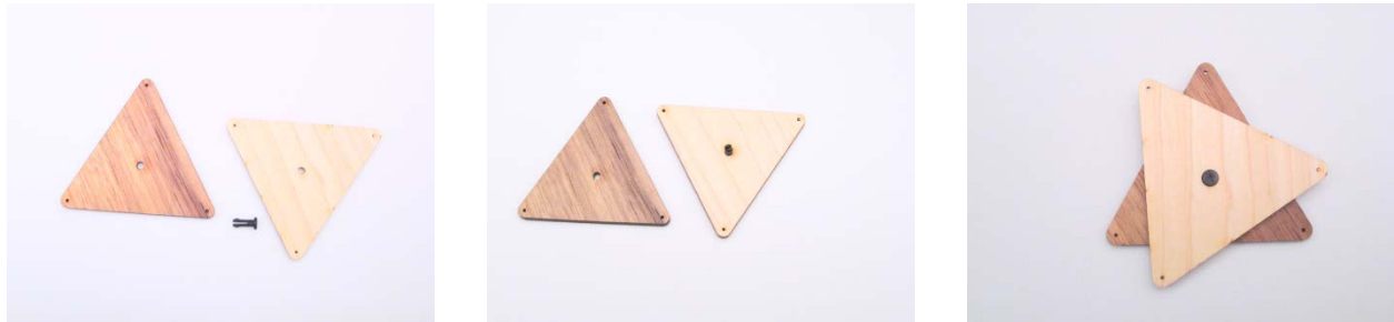
Figure 2: Step one - Two triangles & one rivet assembly.
