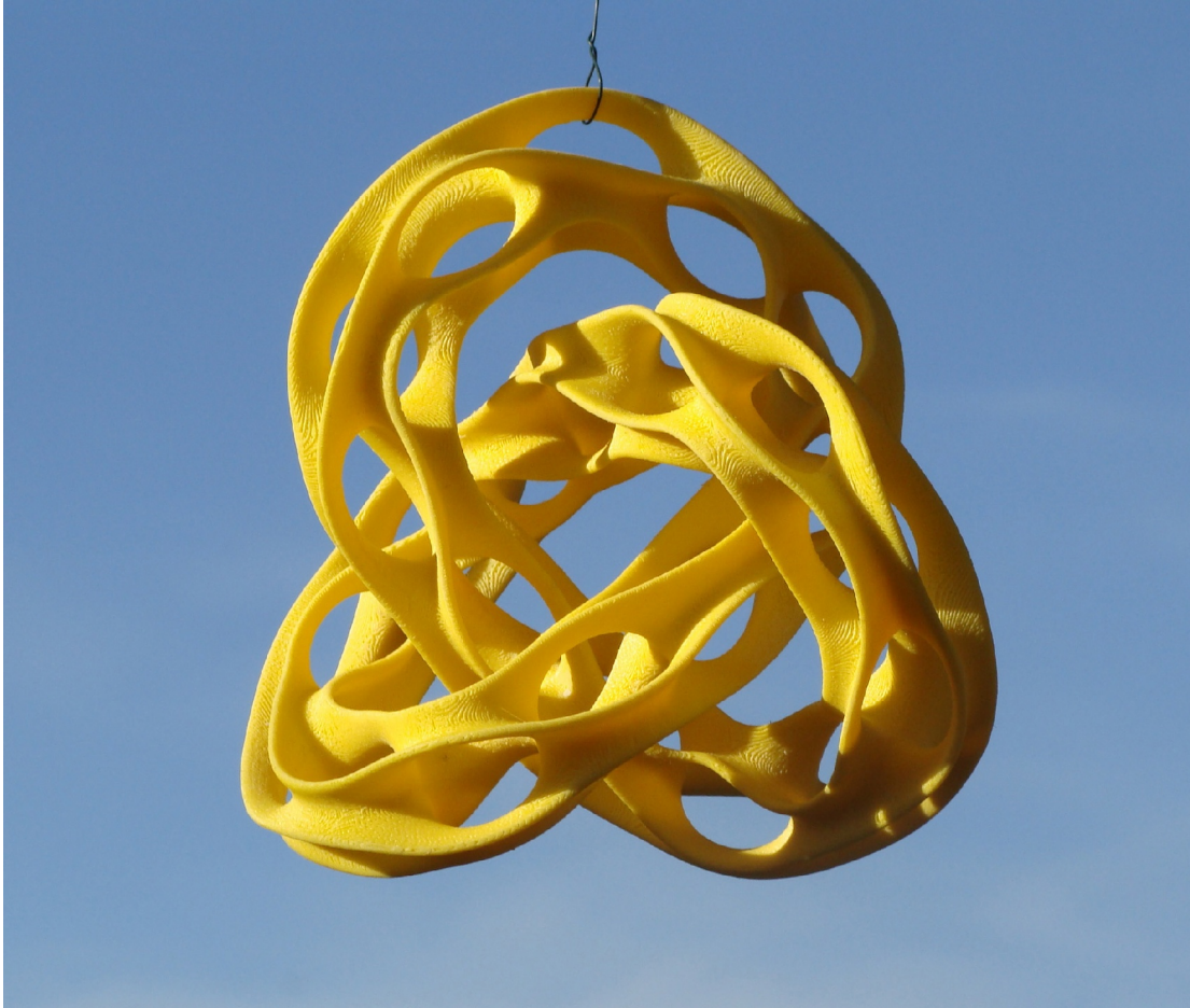
Figure 2: “Evolving Trefoil.” A 7-inch plastic maquette of the final sculpture design, created on a fused deposition modeling (FDM) machine. The geometry description for this model [3], produced by Carlo H. Séquin at U.C. Berkeley is also used in a numerically controlled milling machine to fabricate the master geometry module for making a mold to cast this 12-foot diameter sculpture from six identical pieces.
