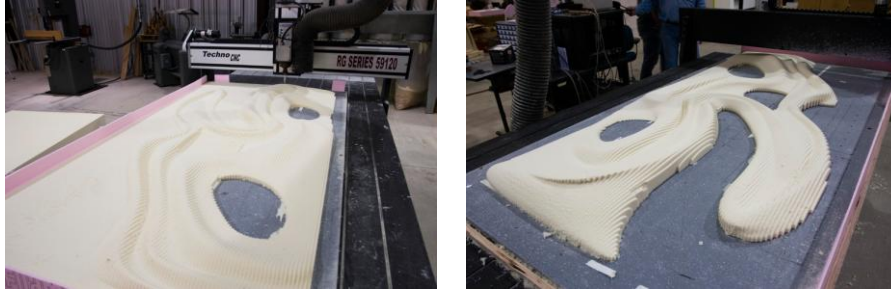
Figure 3. Photographs showing the first, second step-down of the rough cut, a detail of the rough-cut and the finish-cut. The complete installation required a total of 8 sheets of 2 lb. foam and 2 sheets of 10 point foam were employed depending on structural requirements inherent to each segment, see figure 2.
