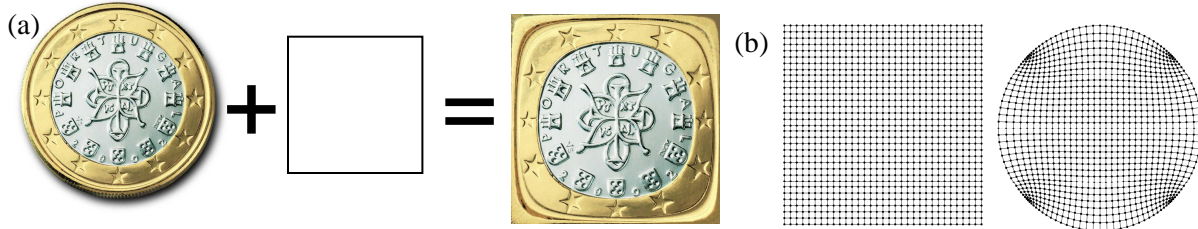
Figure 4: (a) Given an image (of a euro) and a target shape (square), map the image of the euro to the square. (b) An inverse mapping that accomplishes this.
