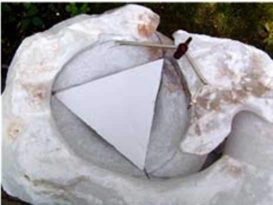
Figure 26 and 27 Calculating the locations for the split using an equilateral triangle. Miscalculation leads to almost irreversible non-parallel paths.
