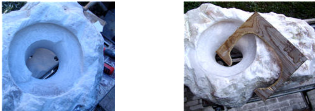
Figure 22 Finishing the inner curvature using carton stands Figure 23 Making the outer curvature of the torus using a wooden stand.
