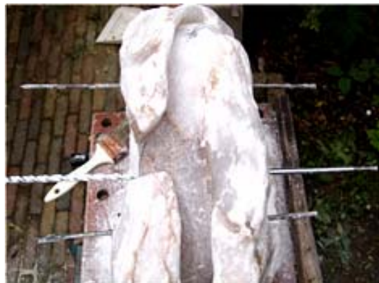
Figure 26 and 27 Calculating the locations for the split using an equilateral triangle. Miscalculation leads to almost irreversible non-parallel paths.
