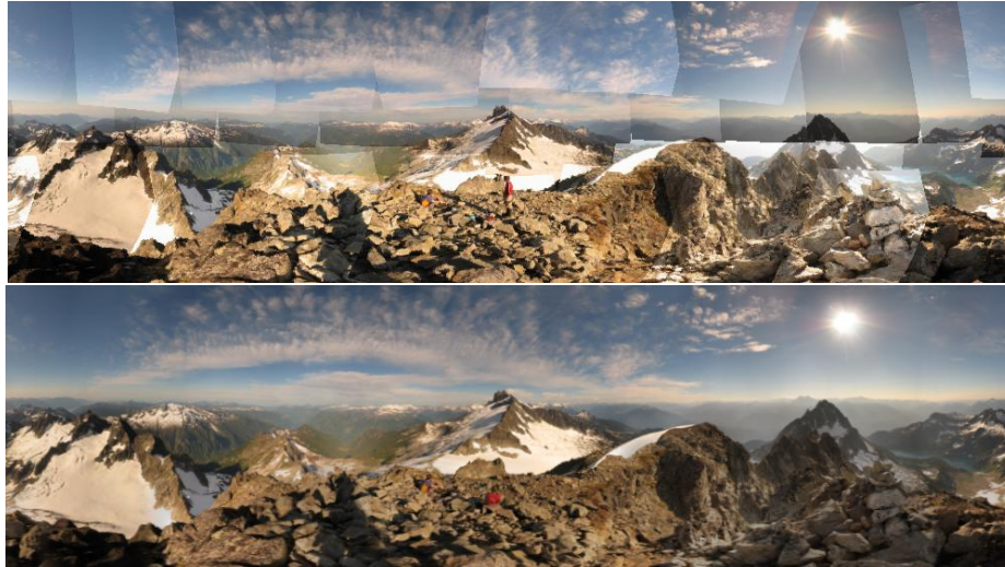
Figure 1: To stitch a collection of images pairwise, first their SIFT features are computed, then the ones appearing in both images are obtained. The optimal transformation for mapping these points is applied to the second image, yielding partially overlapping images. Blending is used to optimise the colours. Figures taken from the Autostitch web site.
