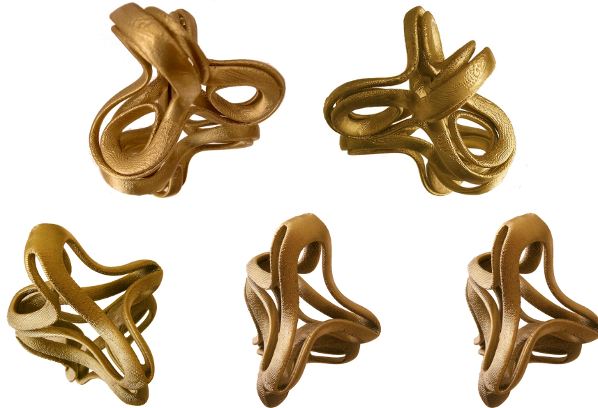
Figure 1: 3D prints of the models created in TopMod. For each sculpture, we took two photographs from slightly different point of views. The sculptures are photographed on a mirror. Background is eliminated. These shapes are made from ABS plastic and printed using a Fused Deposition Machine (FDM). They are later painted using an acrylic paint. The ribbon shape on the left is really a genus-1 surface, but, during the construction of this surface, genus changed several times.
