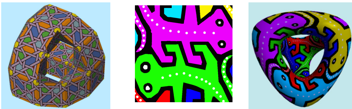
Figure 13: Texturing the tetrus. A polyhedral tetroid suitable for Catmull Clark subdivision (a); a quadrilateral tile with two “newts” (b), and the result of texture-mapping it onto a tetrus (c).
