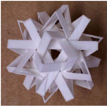
Figure 17. 10 triangle SLS model, based on icosahedron.
