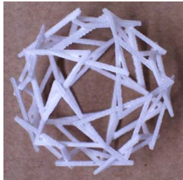
Figure 18. 20 triangle SLS model, based on icosahedron.
