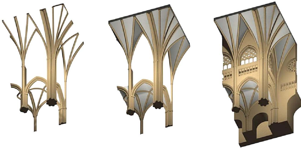
Figure 3: Interior of the Bilbao Cathedral. The making of a computer model is similar to the physical creation of the Cathedral. First, the columns and arches are constructed, followed by the vaults, piers and flying buttresses, and finally the walls, windows and ornaments.
