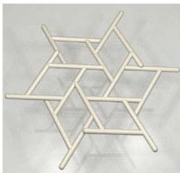
Figure 27: Leonardo grid 2D. grid 3D.
