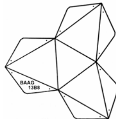
Figure 14: Star pattern with 1/3 triangles, position and color coding plus drill holes.
