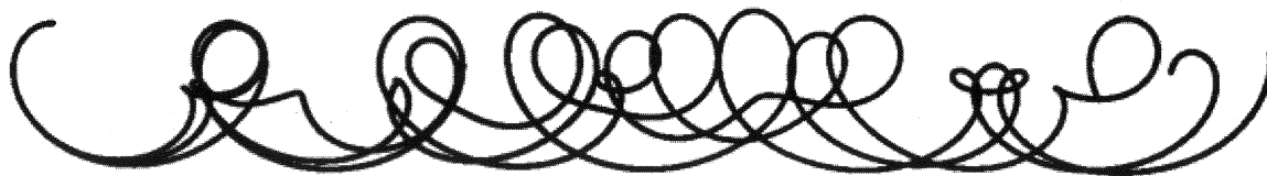
b) Paths of the top vortex for three different time steps. Figure 7: Simulation of chaotic leapfrogging with three ring vortices.
