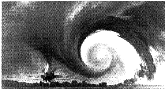
Figure 1: Wing tip vortex [2].
